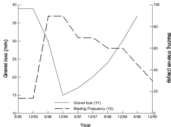
**FIGURE 1: Gravel loss and blading interval over time**
