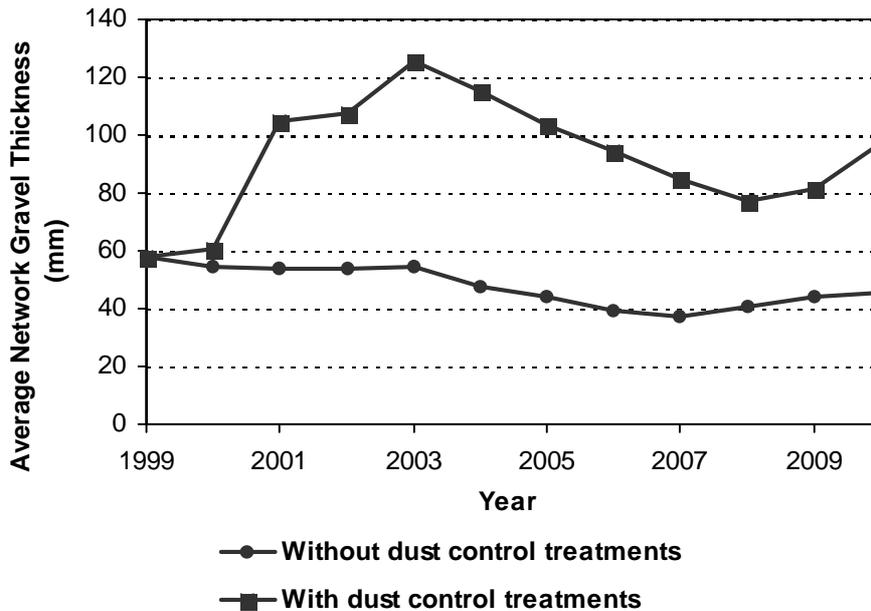
**FIGURE 2: Predicted average network gravel thickness**
